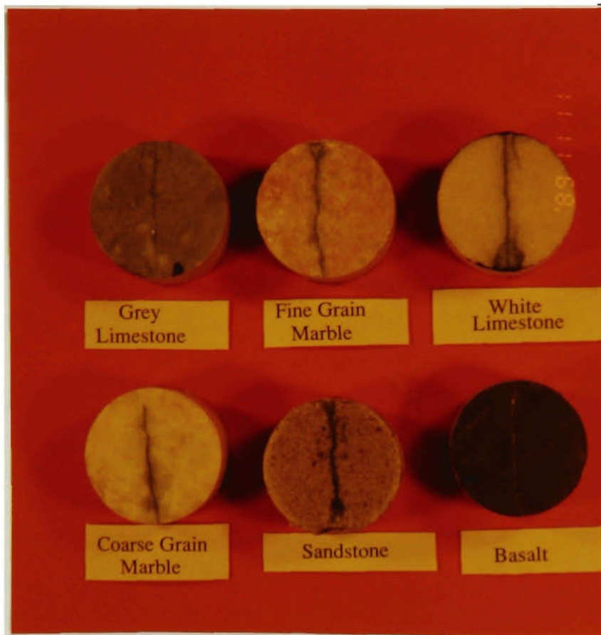
Figure 6.9 The fractured specimens after Brazilian tests
